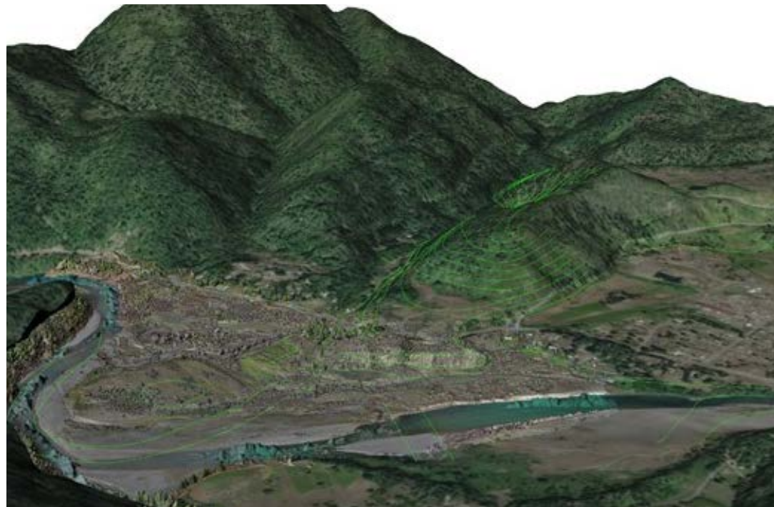
Figure 3.8 Rhino model of Tishánik with historic contours overlaid in green to visualize land loss from hydraulic mining
