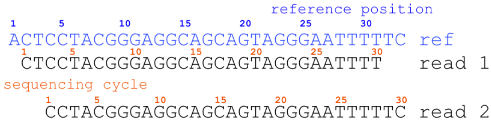
Figure 4.6: Sequencing cycle versus reference position. Our reads didn't always start at the first base of the primer region. We use sequencing cycle to refer to the position on the read and reference position to refer to the position on the MP/DR sequence.
