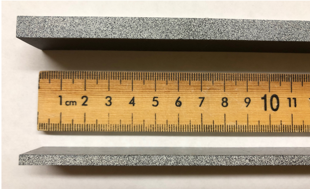
Figure 2.3: Beam speckle shown on an approximately 8 mm thick specimen (top), and on an approximately 4 mm thick specimen (bottom)
