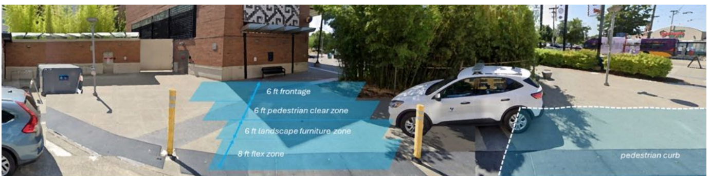
FIGURE 3-25. CROSS SECTION DETAIL OF TEAM 1 SOUTH (WEST END); SOURCE: ADAPTED FROM GOOGLE STREET VIEW
