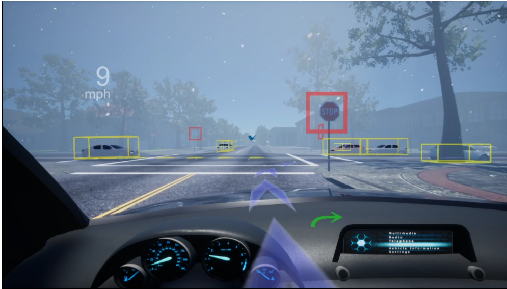
Figure 3.1: An example screenshot of the study scenario of low visibility and high automation transparency. The bounding boxes highlight the signs, cars and other moving objects in sight.
