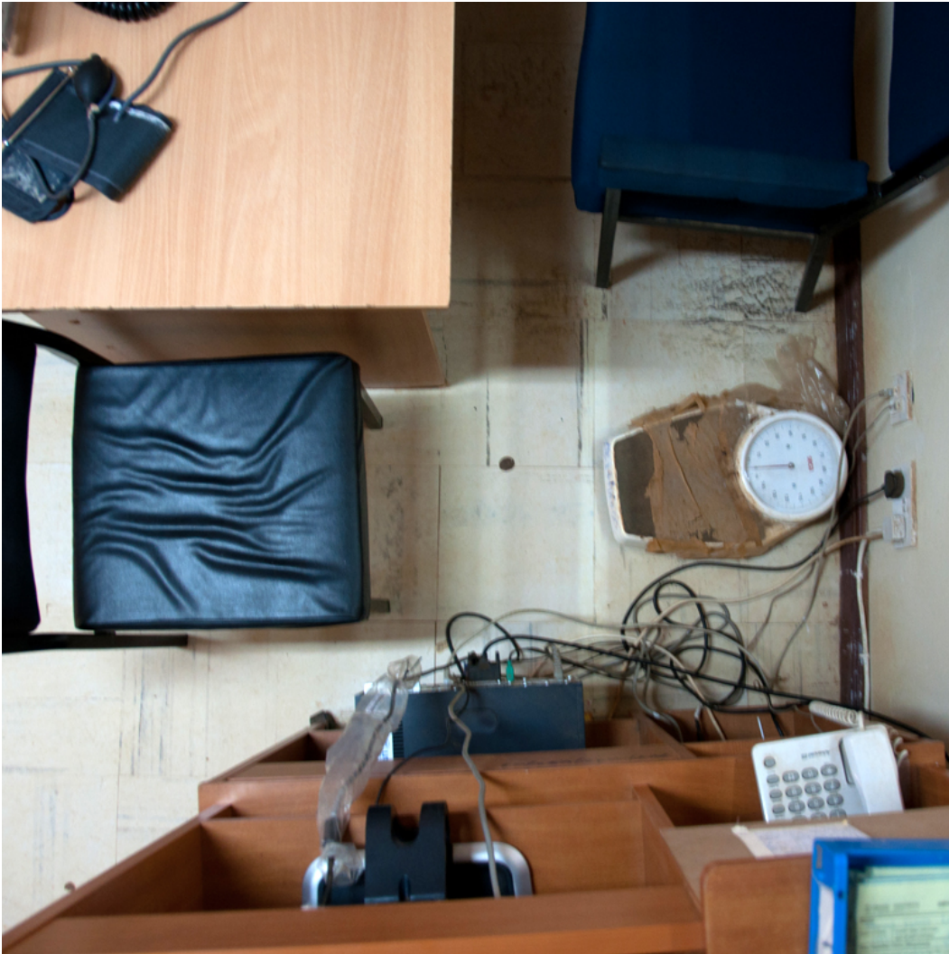
Figure 3.8: In this view of a clinic (looking down from the ceiling), the nurse sits in the right chair, and the patient sits on the left. The patient's feet (or her young children) might accidentally disconnect the cables and disable summary printing. Because of a lack of technical ability and power dynamics at the clinic, weeks often pass before such problems are properly diagnosed and reported to supervisors.
