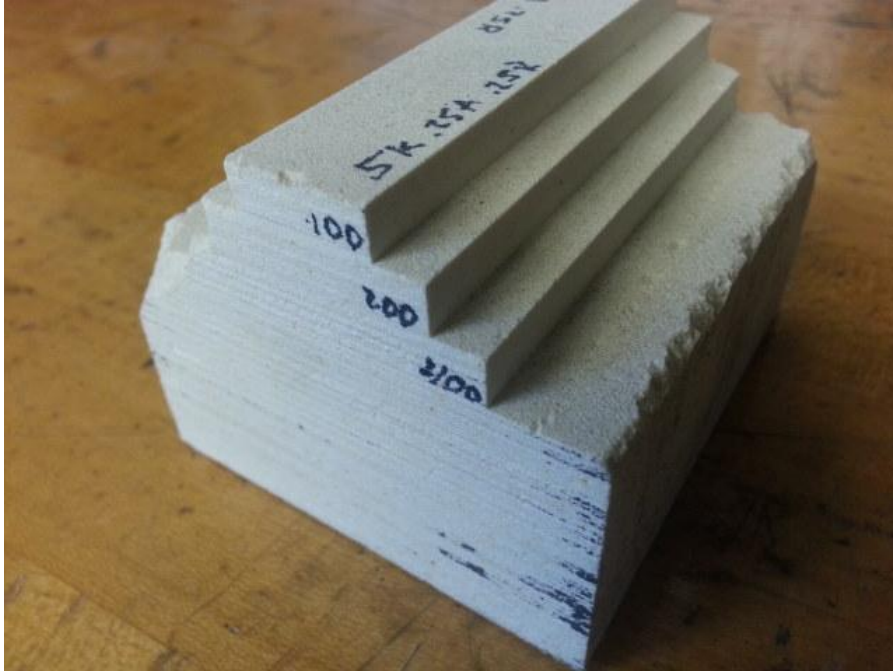
Figure Q-487: CB1100 surface roughness sample.
