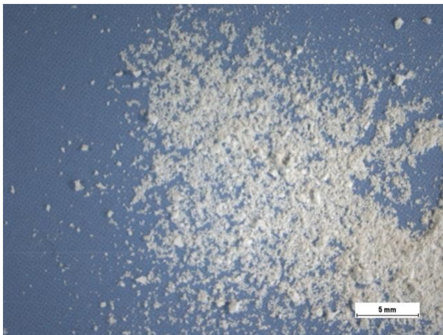
Figure 6-1: Typical dust collected while machining AAC
