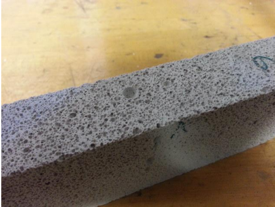
Figure Q-497: AAC four point bend specimen.
