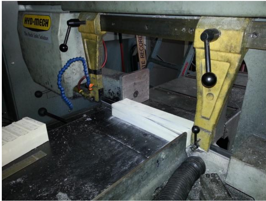
Figure Q-477: Horizontal bandsaw cutting CB1100 blocks
