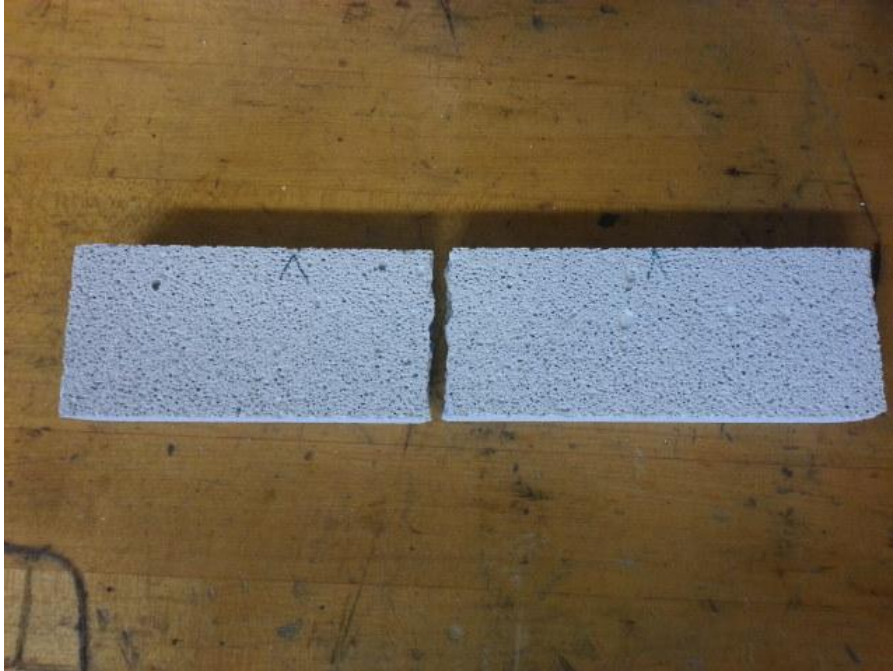
Figure Q-493: Fractured AAC four point bend specimen.
