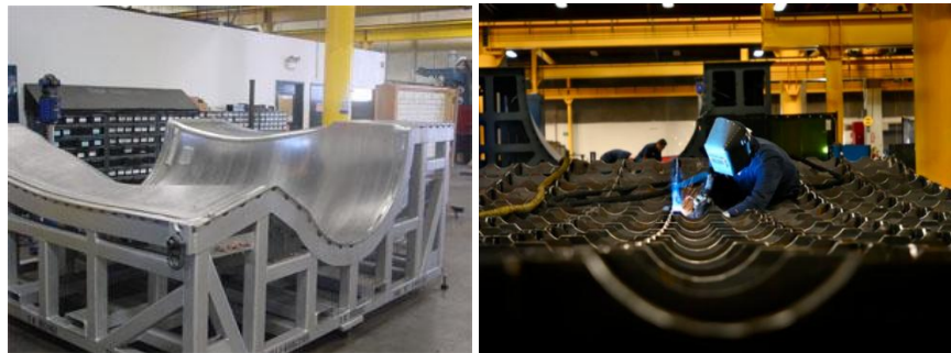
Figure 1-1: (a) Example of a metallic based composite layup tool [5] with (b) bottom view of a large metallic tool substructure [6].
