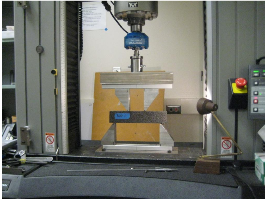
Figure Q-505: Photo image of Cfoam four point bend testing.
