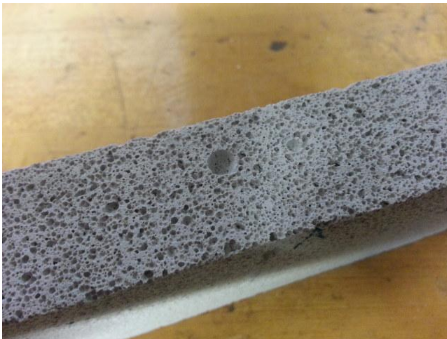
Figure Q-495: Fractured AAC four point bend specimen.
