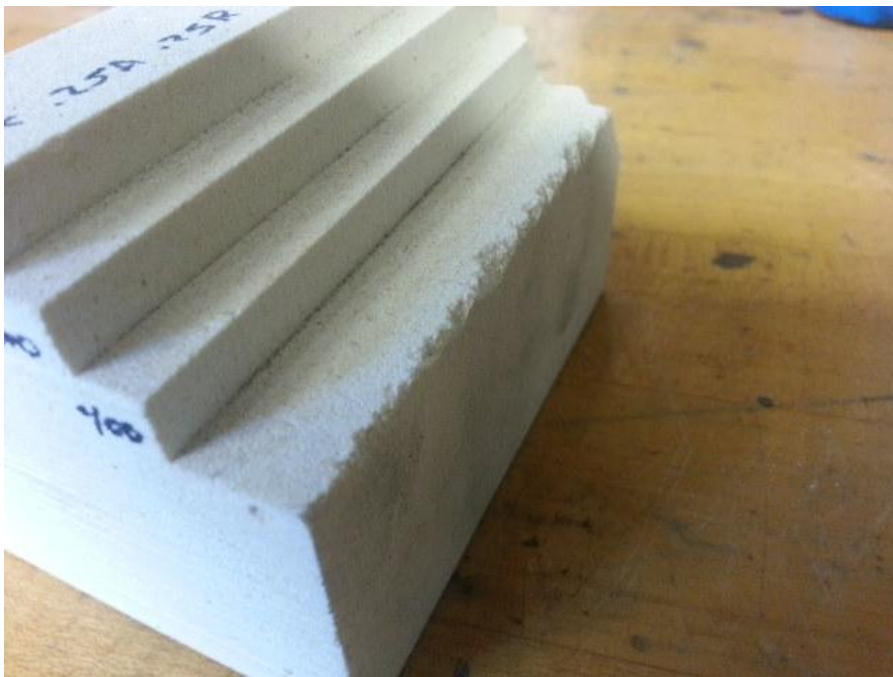
Figure Q-485: CB1100 surface roughness sample.
