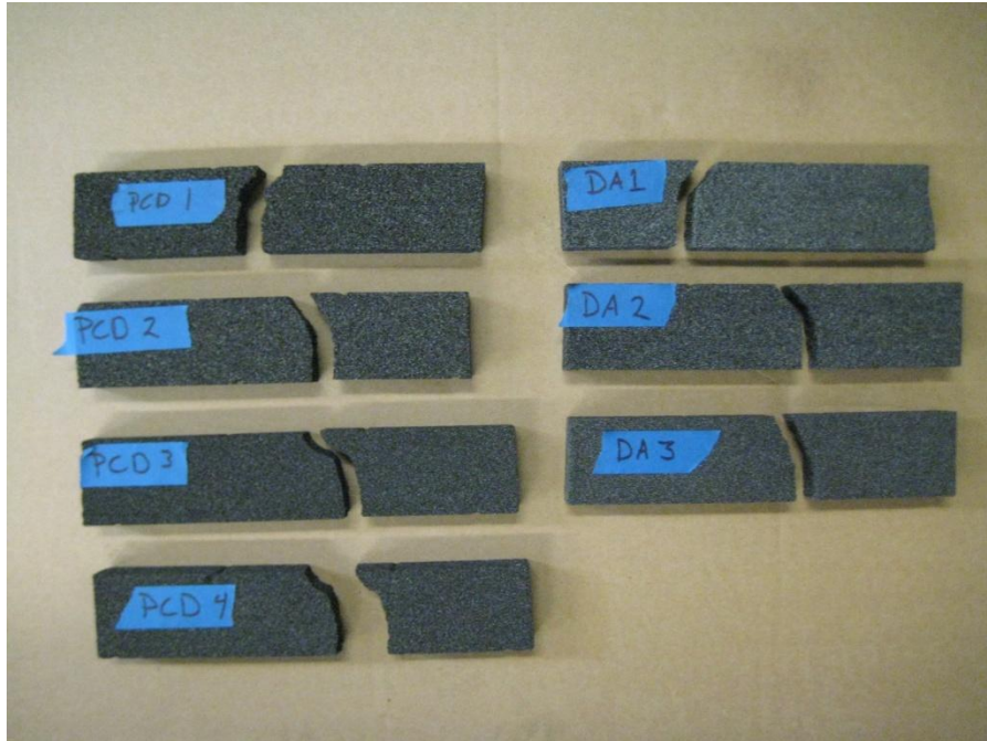
Figure Q-499: Fractured Cfoam four point bend specimens.
