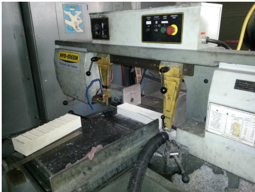
Figure Q-478: Horizontal bandsaw cutting CB1100 blocks
