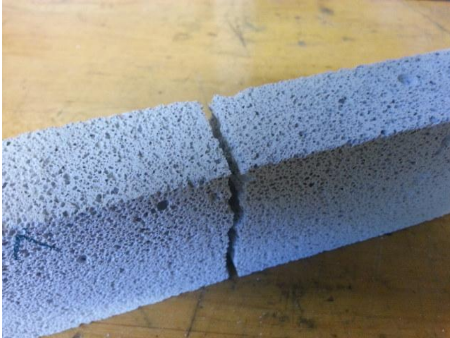
Figure Q-495: Fractured AAC four point bend specimen.
