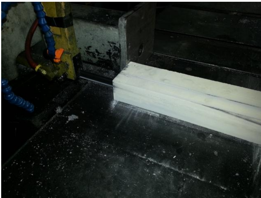
Figure Q-480: Horizontal bandsaw cutting CB1100 blocks
