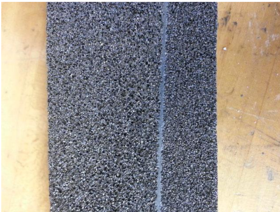
Figure Q-498: Photo image of bonding line in Cfoam.
