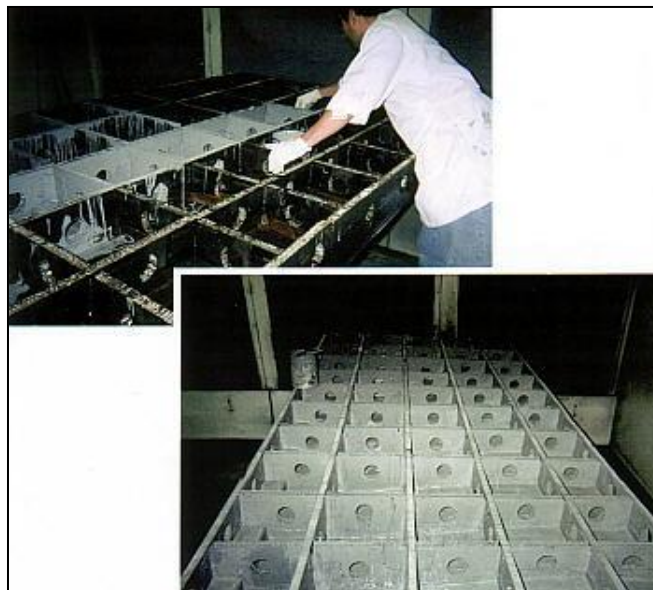
Figure 1-2: Example of composite based layup tool "egg-crate" backup structure made from CFRP [23].
