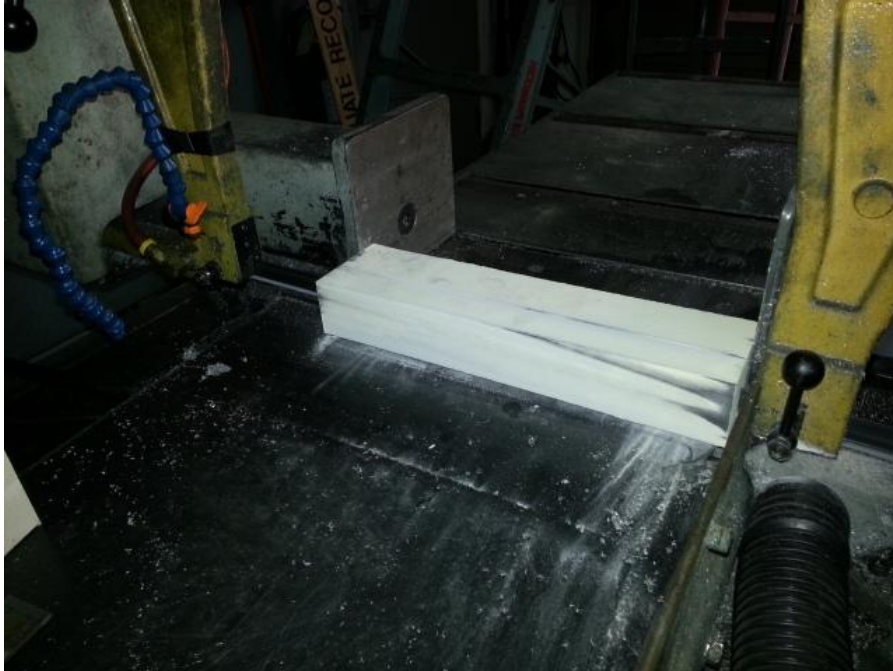
Figure Q-479: Horizontal bandsaw cutting CB1100 blocks
