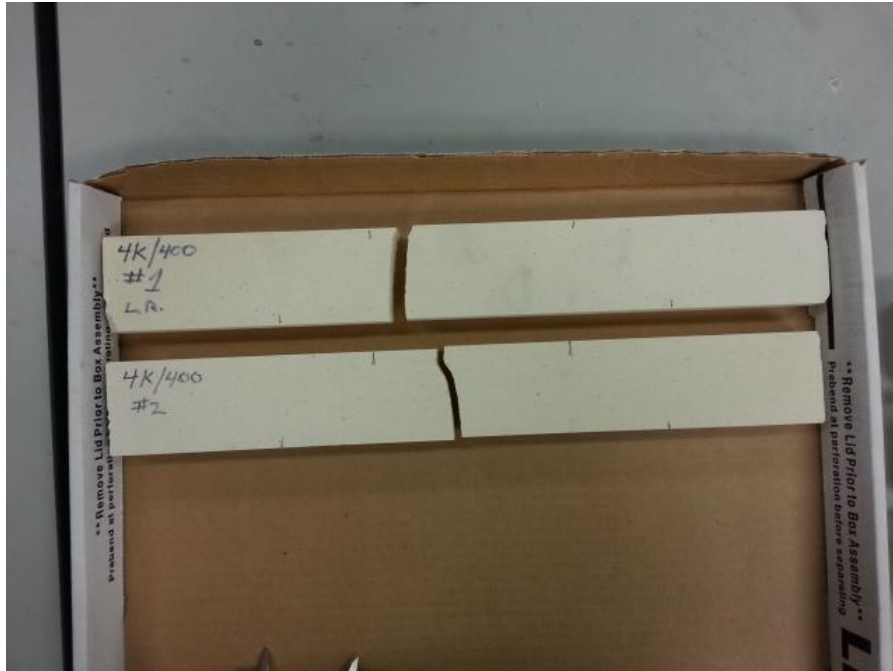
Figure Q-491: Fractured CB1100 four point bend specimens.
