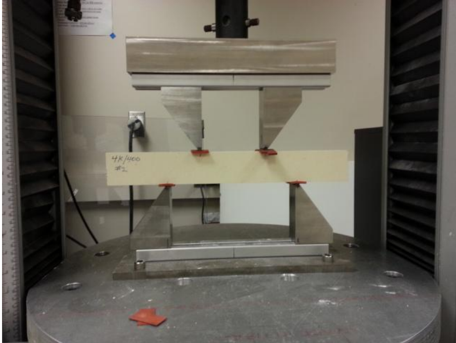
Figure Q-483: CB1100 four point bend specimen in fixture.
