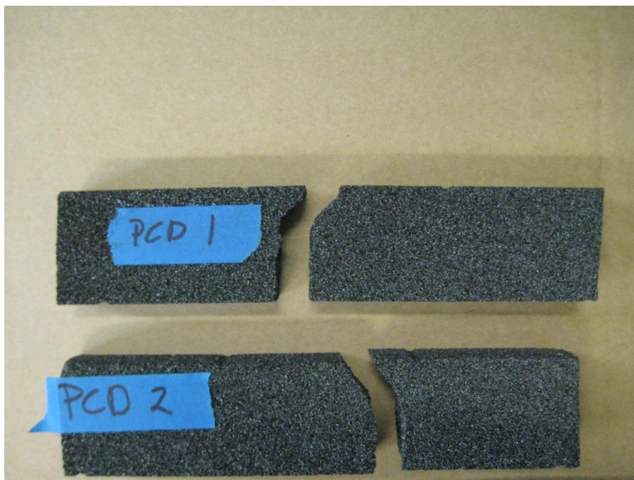
Figure Q-501: Fractured Cfoam four point bend specimens.
