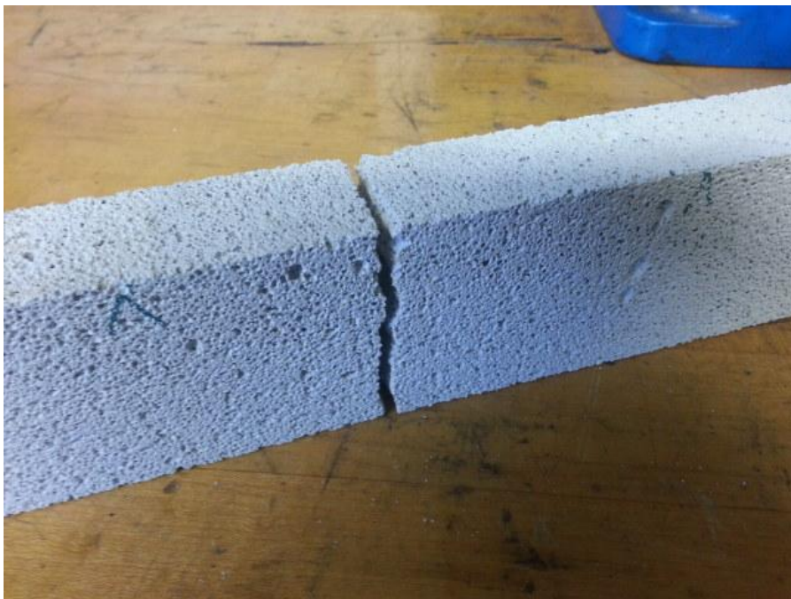
Figure Q-493: Fractured AAC four point bend specimen.
