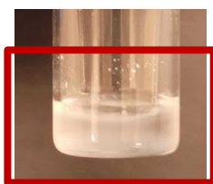
Figure 3.7 Sample composed of the 80 mol% Choline Chloride with Acetamide. The sample was heated using a hotplate and formed an opaque solution, which is a sign of formation of two phases.
