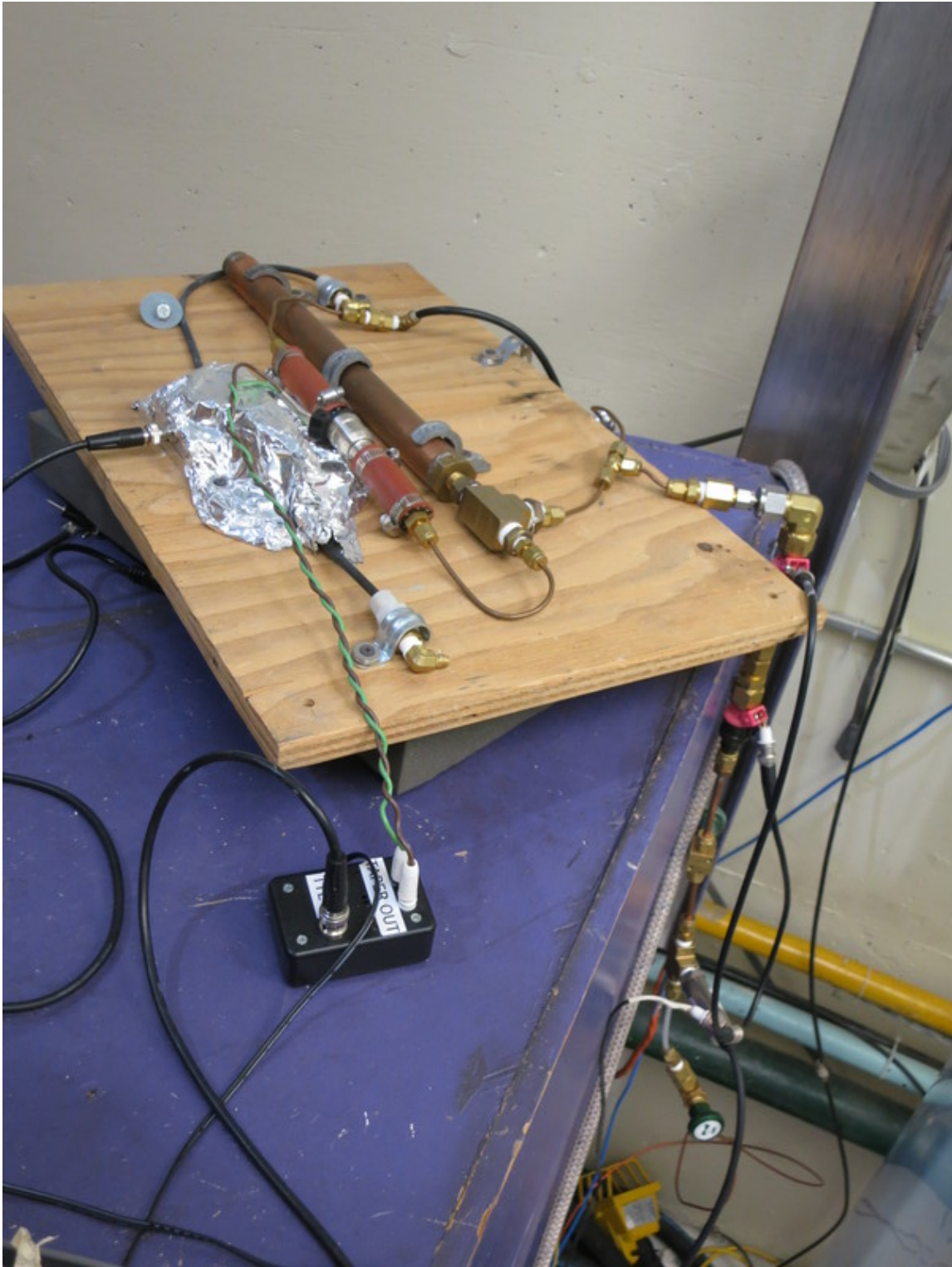
Figure 2.19: The gas-handling system. It is remarkable that a system with such a crude appearance can yield such good performance. Low leaks, a high-precision gauge, and the three reliable/fast automotive fuel injectors are key to its performance.
