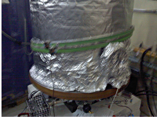
Figure 9.2: Coil in the on-apparatus position. Current was applied to the coil in both directions, allowing searches for systematics proportional to both \vec{B} and |\vec{B}|^2 .
