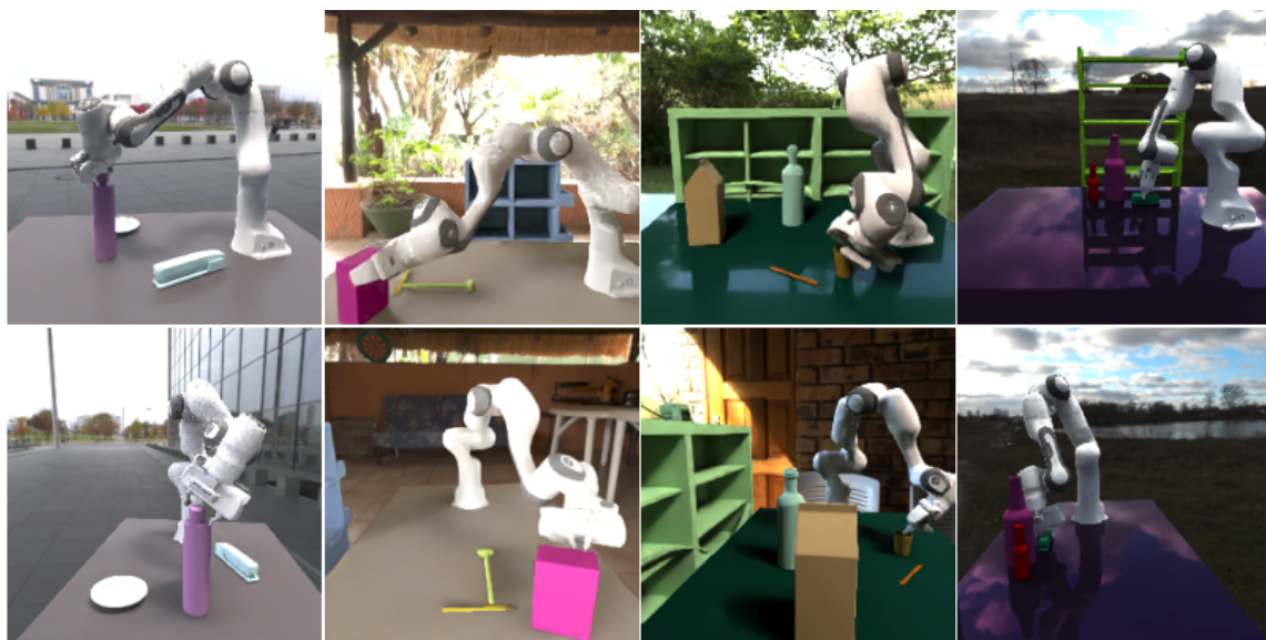
Figure 2.6: Sample scenes from the kitchen dataset. The top and bottom rows show two different views. SORNet can leverage additional views to improve performance, but does not require multiple views.
