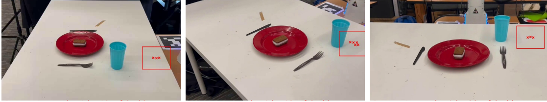
Figure 4.4: RoboPoint’s prediction is consistent across different viewpoints. Red cross shows RoboPoint’s response to “find free space right of the blue cup” in different views.
