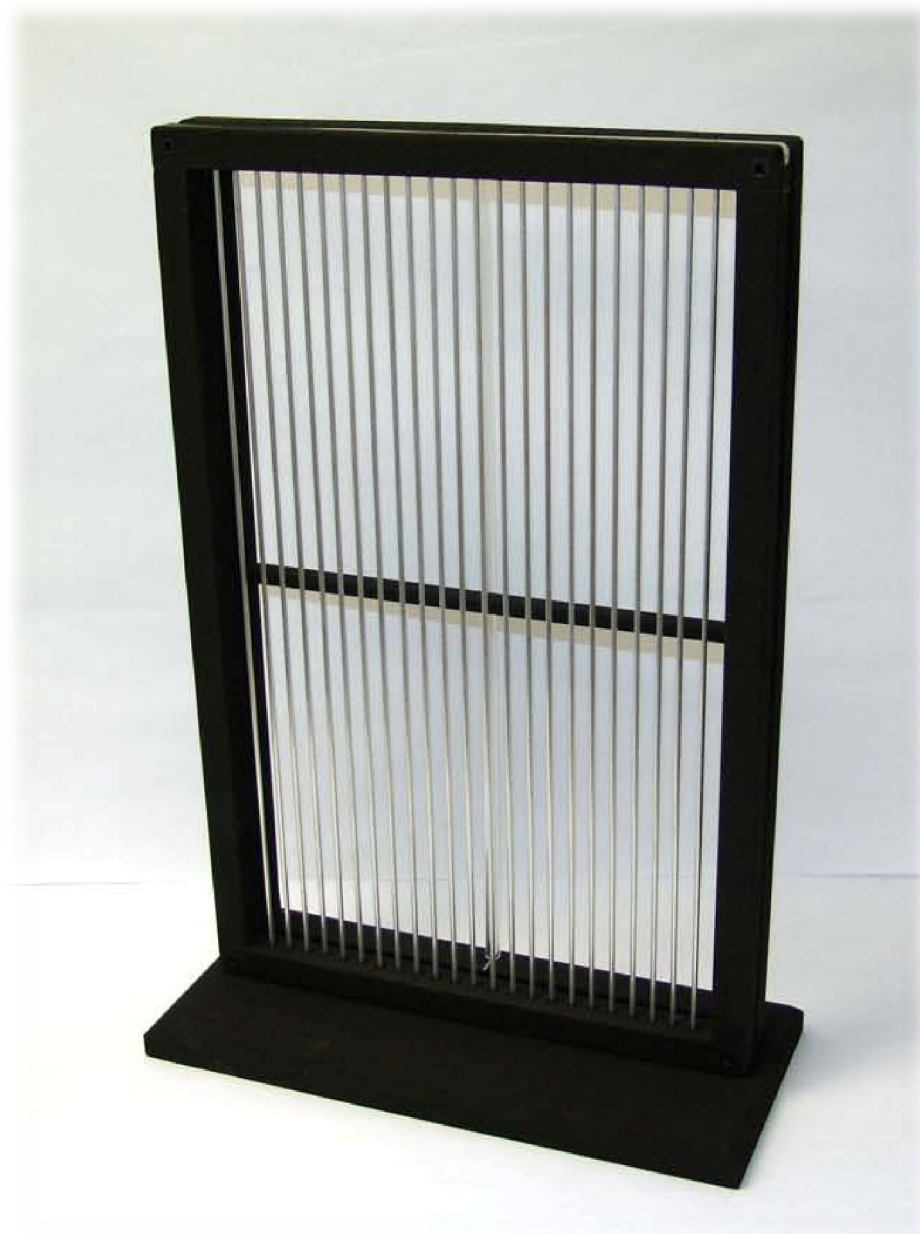
Figure 8.2. Single Kronos EHD loudspeaker shown without an enclosure, fabricated from two parallel arrays of collector and emitter electrodes made from thin Al rods and 100 \mu\text{m} diameter W wires respectively.
