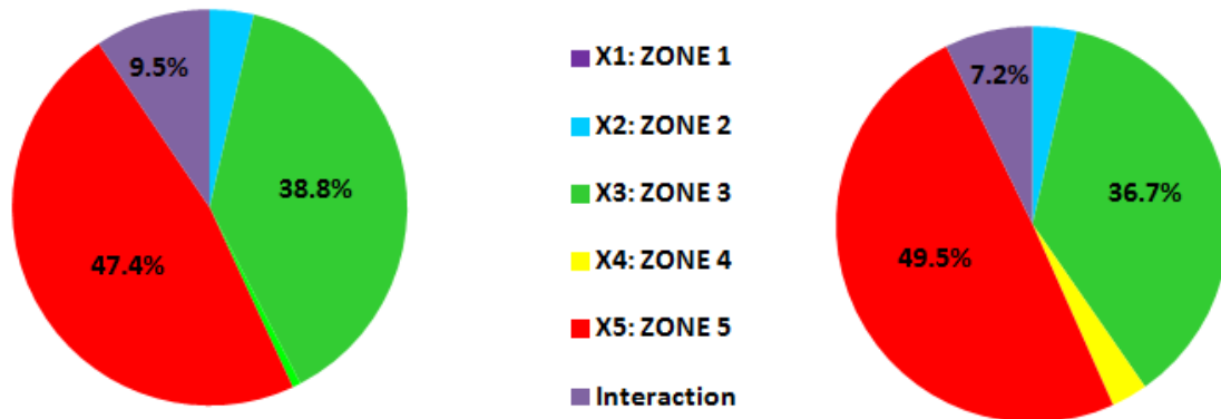
Figure 4.29. Flutter index and frequency sensitivity to zone discretization for the M=0.954 case
