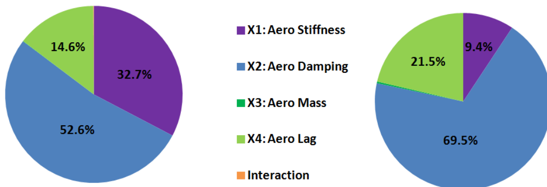
Figure 4.32. Flutter index (left) and flutter frequency (right) sensitivity to Roger terms for the M=0.954 case
