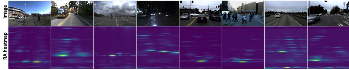
Figure 2.11: 8 scenario examples in the collected UWCR dataset: rows 1, 3 are the camera images; rows 2, 4 are the corresponding radar Range-Azimuth angle heatmaps.
