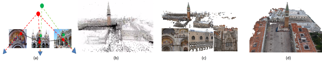
Figure 2.1: (a) shows the triangulation process of bundle adjustment, where detected and matched features across images, are used to recover the camera parameters shown in (b) for the San Marco data set, computed using [9]. Each black dot show a reconstructed cameras. (c) shows the result for [35] for the San Marco data set. The top image shows the entire reconstruction whereas, the bottom layer shows us zoomed in regions. (d) shows the result for the approach in [87], using aerial streetview photography as well.
