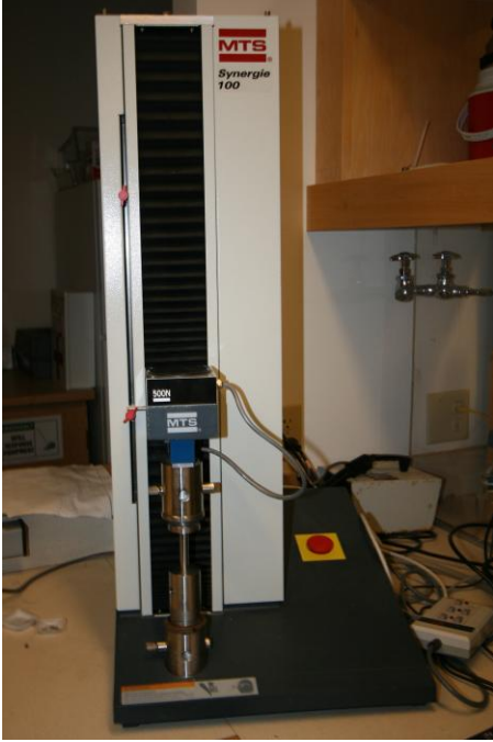
Figure 5. MTS Synergie 100 crushing machine with digital force gauge used to measure peak force (N) when breaking limpet shells
