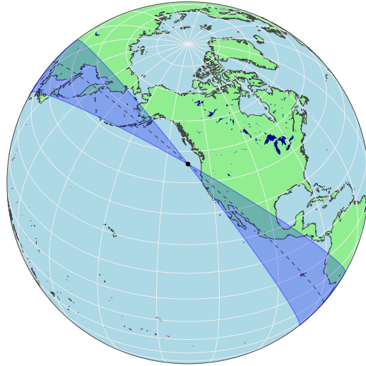
Figure 3.2: Endfire bearings \pm 10^\circ for the Central Caldera and Eastern Caldera hydrophones.
