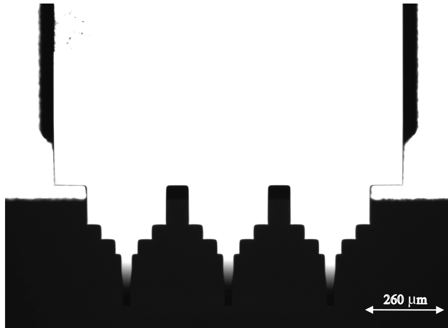
Fig. 7. Microtip surface capture with an optical microscope at 4X magnification
