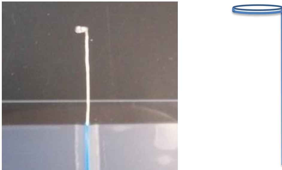
Fig. 14. Aluminum coil for 5ul solution droplet
