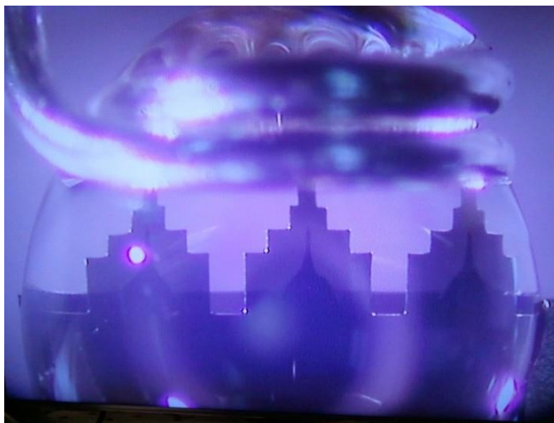
Fig. 18. Microtip inserted into coil with solution droplet so that the end of the tips are underneath the middle of the wire coil.
