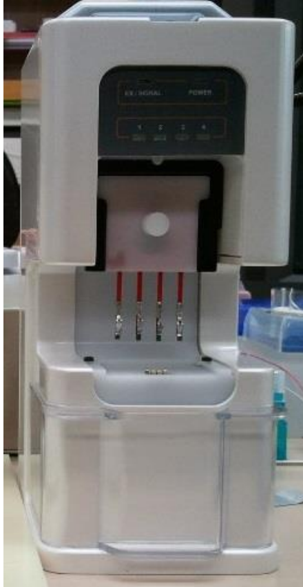
Fig. 21. Nanofacture Incorporated automated DNA purification device prototype.
