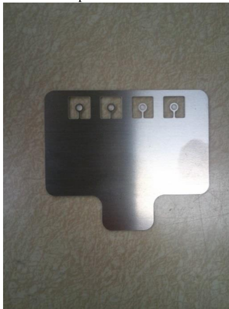
Fig. 20. Automated device coil plate. In practice these pre-manufactured coils were replaced with wire coils taped to the surface and stripped to make electrical contact.
