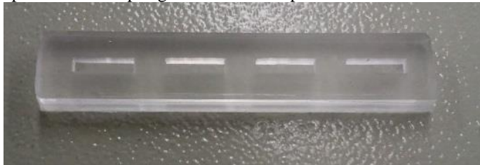
Fig. 10. PDMS wells used to hold diluted PEI solution for microtip functionalization
