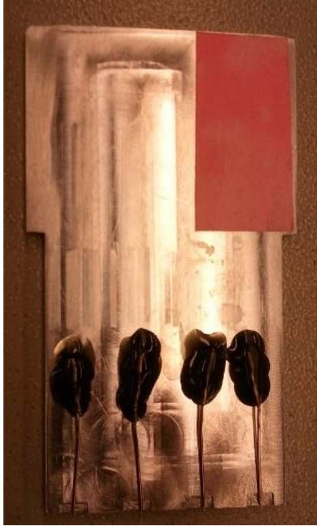
Fig. 9. Aluminum coupon with wire springs to hold microtips in channels at the base of the structure
