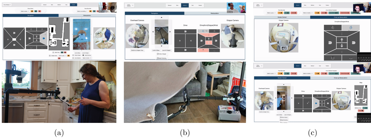
Figure 6.2: Henry’s customized interfaces for (a) handing jam to Jane, (b) playing with his granddaughter, and (c) turning his percussion vest machine on or off.
