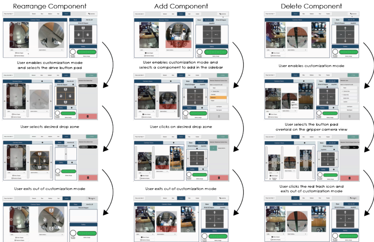
Figure 5.3: Example of how a study participant used the customization mode to (left) rearrange components in the interface, (middle) add a new component, (right) and delete a component.
