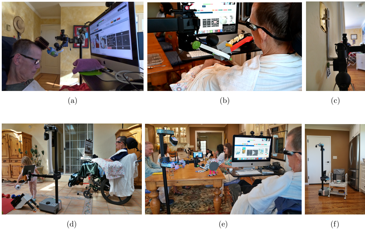
Figure 6.1: Henry Evans completing tasks independently by teleoperating the Stretch RE2 to (a) scratch his itches, (b) feed himself, (c) flip a light switch, (d) play with his granddaughter, (e) play poker, and (f) tow a meal cart.
