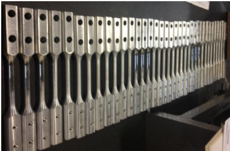
Figure 7-3 Test Specimens - Completed Fabrication
