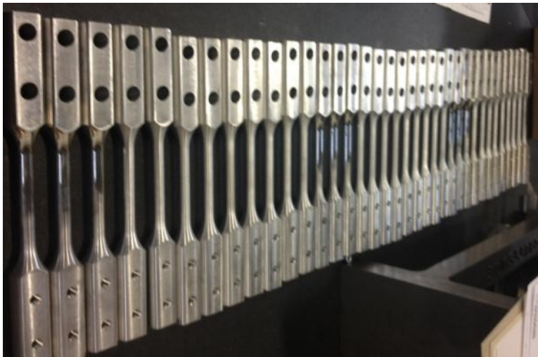
Figure 4-2 Test Specimens - Completed Fabrication
