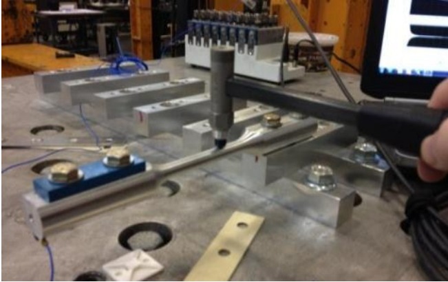
Figure 4-12 Constrained Modal Test Impulse Impact Location
