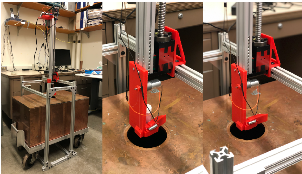
Figure 4-15. Photograph of the automatic sample loading system. Left, the overview of the system setup; Middle, the initial state of the system; Right, the final state of the system.
