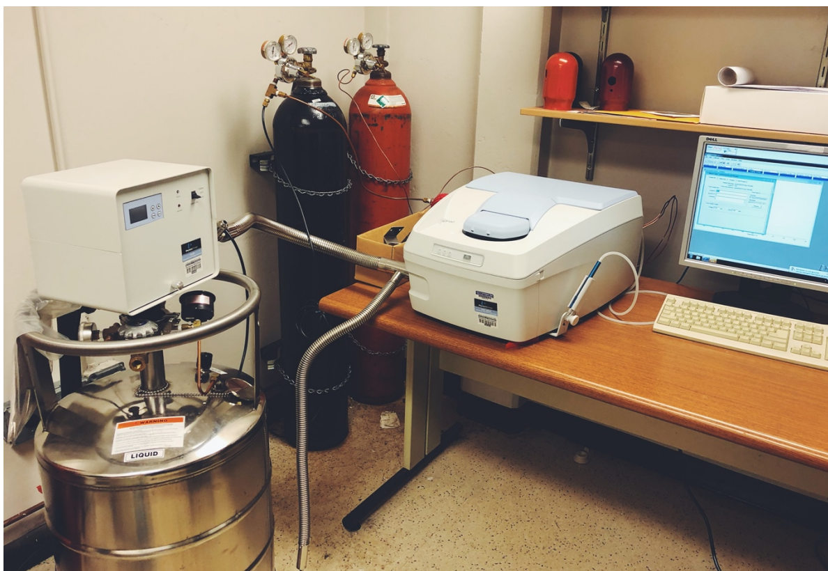
Figure 3-7. The measurement system setup of the heat capacity
