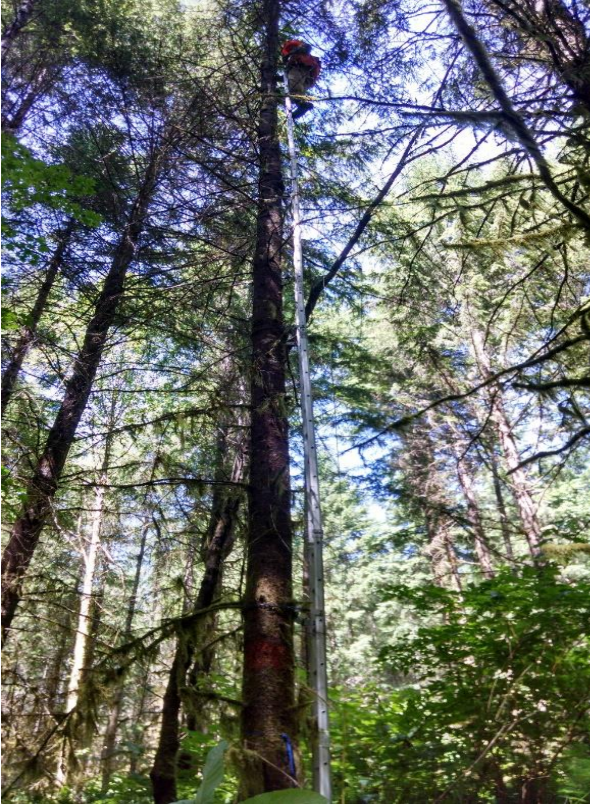
Figure 2A: Swiss-style climbing ladders were used to reach 42' in the canopy of measurement trees, in this case an unpruned control. The ladder combined with a harness was used to safely climb the tree.
