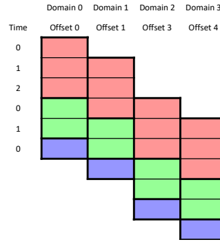
Figure 3.4. Staggering iteration start times across resources.
