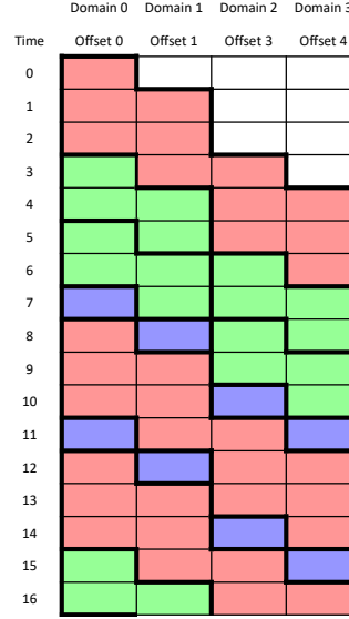
Figure 3.6. Sample Offset Pipelining execution trace of the Figure 3.5 schedule where count is 2, 0 and at least 1 over three iterations of the outmost loop.
