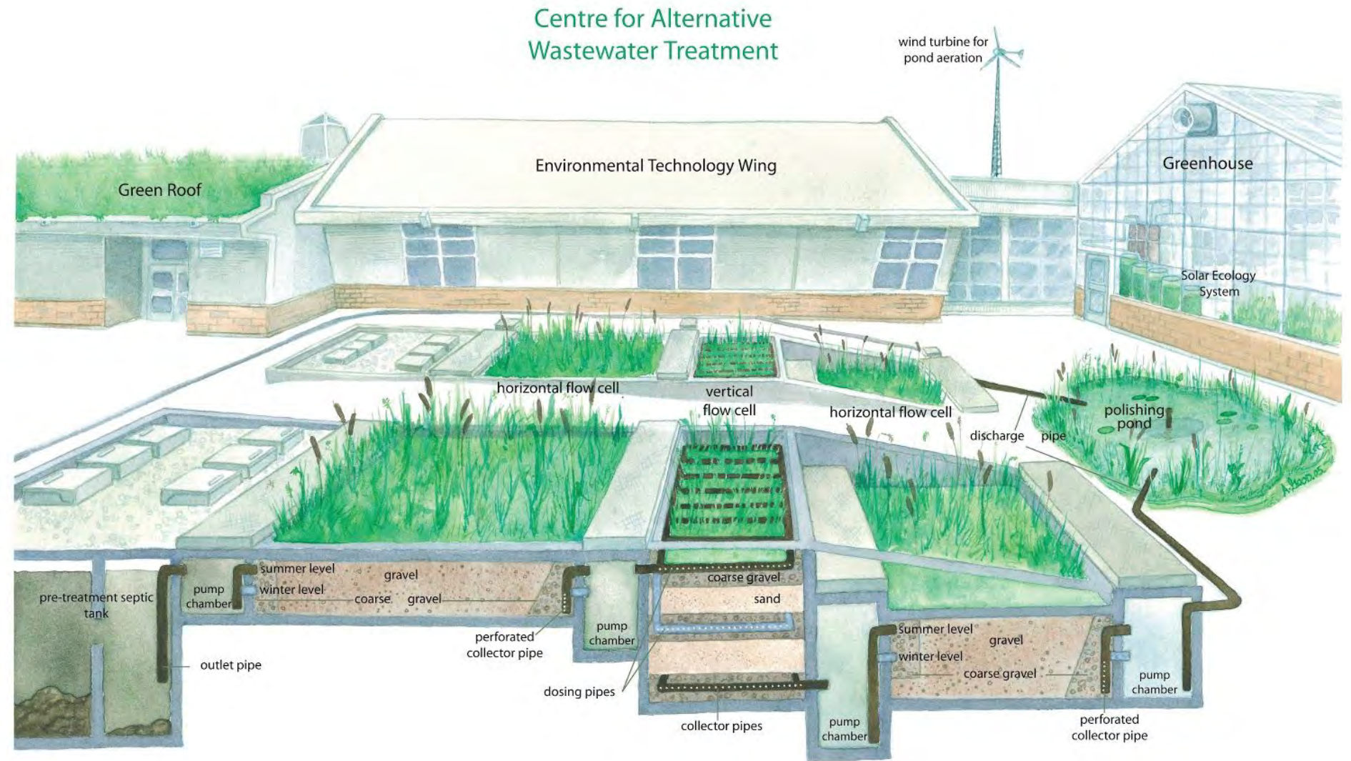
Fig. 68 - Constructed wetlands systems, like the one at Fleming College in Ontario, Canada, comprise an array of different wetlands biomes for the treatment of wastewater. Image: Mclean, 2020.
