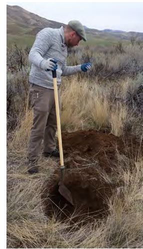
Fig. 125, 126, 127, 128 - It is currently uncertain as to how deep soils run on the proposed construction site before hitting bedrock. Recent test excavations revealed no bedrock at 6' deep.
