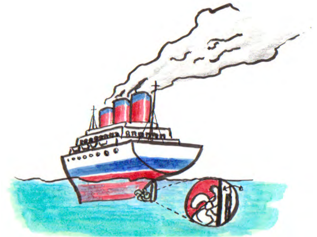
Fig. 1 - An ocean liner with a trim tab. A small push can shift the course of a ship or tilt a planet.
