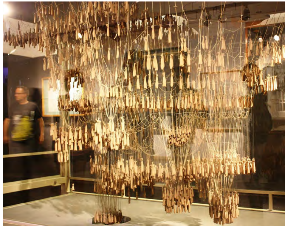
Fig. 58 - A replication of the original model of La Sagrada Família uses weights to distribute loading of catenary arches which form the structure of the celebrated cathedral. Photo: Anne, 2019.
