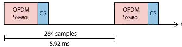
Figure 4.4: FingerIO transmissions at the speaker. The 84 samples for the OFDM symbol and the cyclic suffix are followed by 200 samples of silence. This silence duration is sufficient to receive echoes from all objects within 1 m from the device. Given a 48 kHz sample rate the above transmissions, the above transmissions achieves a frame rate of 169 Hz.
