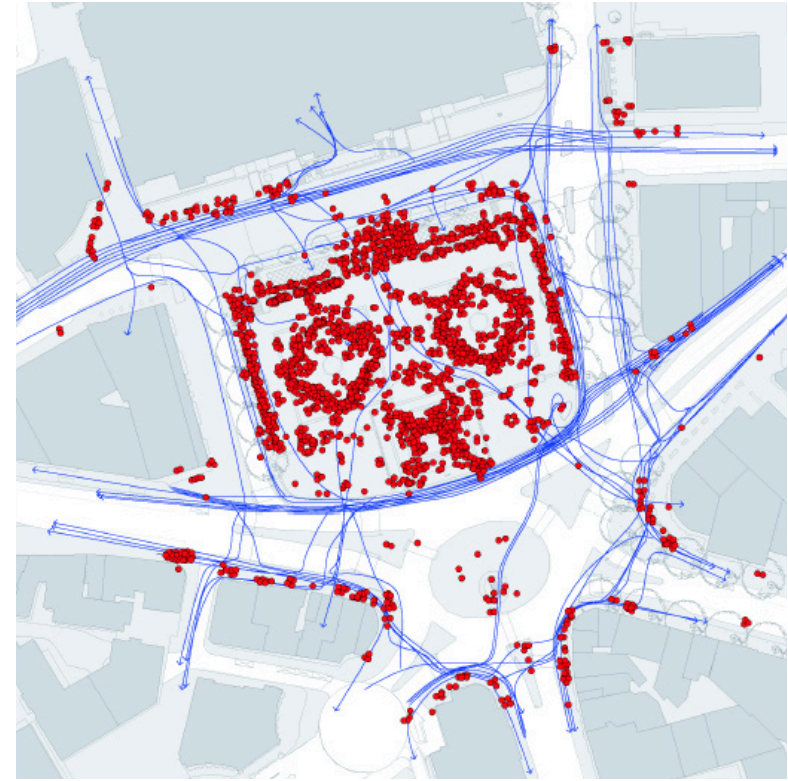
Figure 39 - Space Syntax: Study for Trafalgar Square: Pedestrians after intervention: red dots = dwelling / blue lines: walking.
