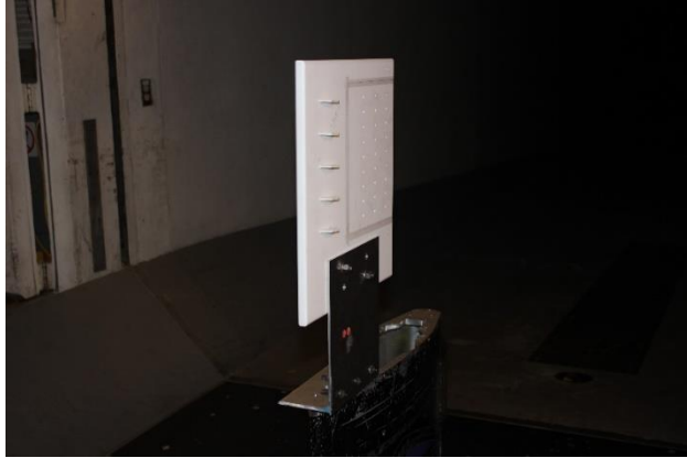
Fig A-ii.3: Plate with 5 VGs mounted in KWT for Iteration 2: Front view
