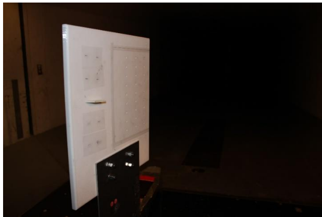
Fig A-ii.4: Plate with 1 central VG mounted in KWT for Iteration 2: Front view
