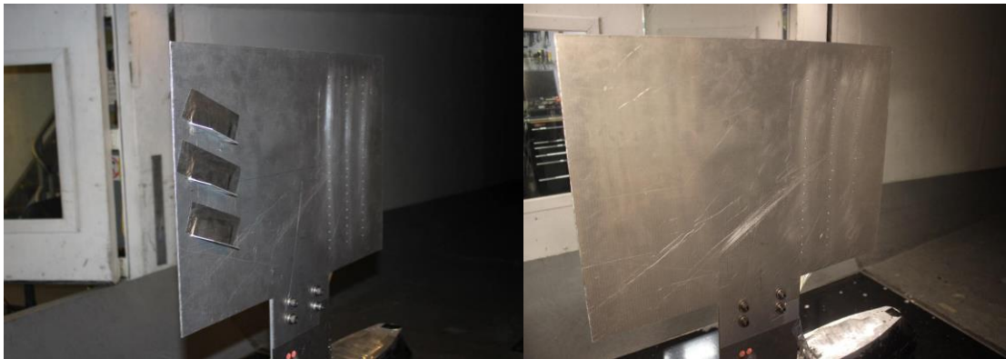
Fig 3.14: Plate 1 with (left image) & without (right image) VGs: Front view
