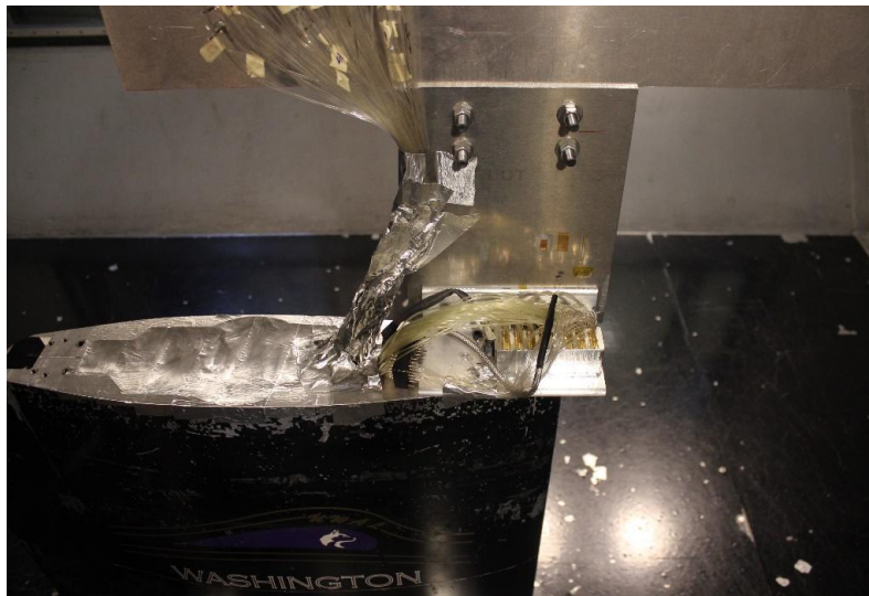
Fig 3.17: Plate Mounting: pressure ports connected to the EPS. The sensing system is placed inside the tunnel mount
