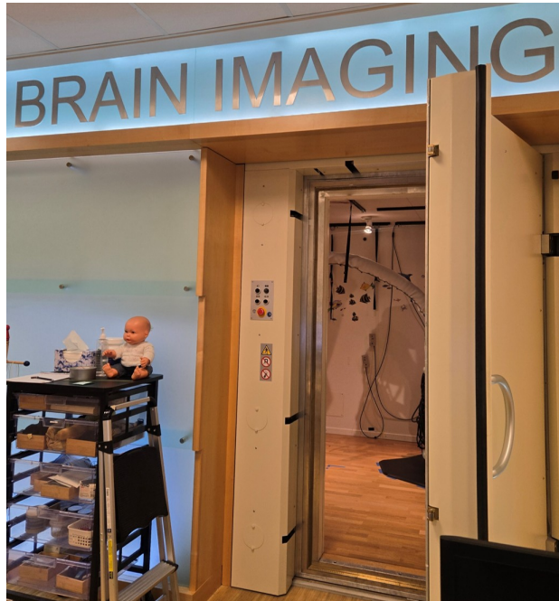
Figure 2.3: The MSR located in the MEG center of I-LABS at the University of Washington. The walls are very thick to accommodate the layers of passive and active shielding. The door is shielded with the same technology and is closed using vacuum technology.
