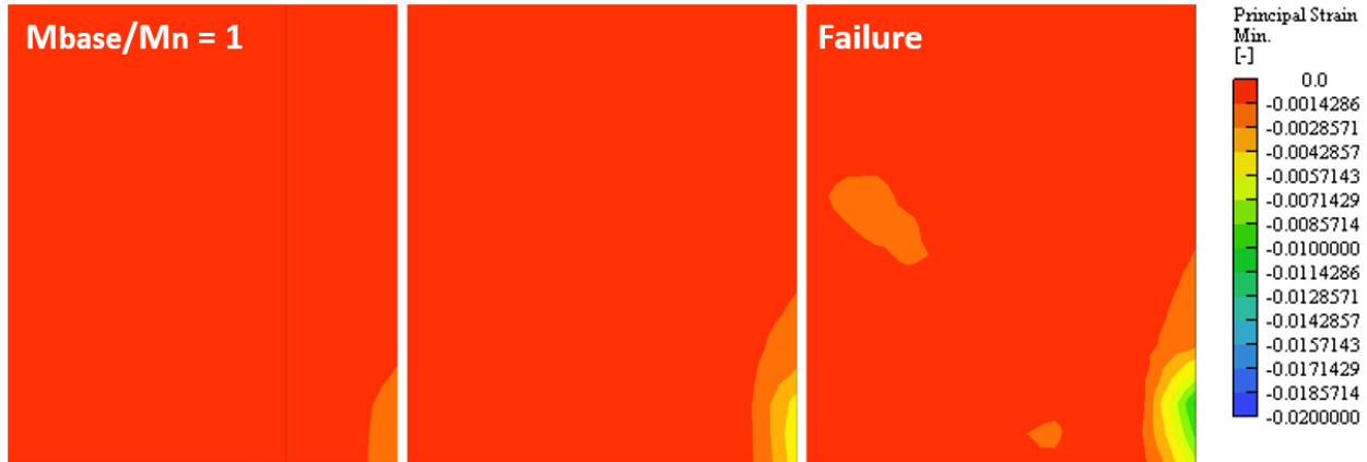
Figure 4.19 – Specimen R1 Min. Principal Strain Contour Plots (Showing Bottom-Right of Wall at 17% of h_w and 36% of l_w )
