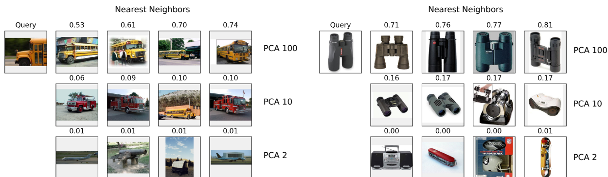
Figure 2.1: A pair of sample queries from the Caltech-256 dataset, showing the four nearest neighbors in three different feature spaces. Each neighbor is annotated with its Euclidean distance to the query in that space.
