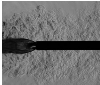
Figure 14: Instantaneous images of (left) Retronozzle Jet Expansion, (right) SRP still image
