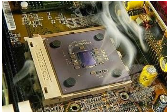
Figure 3: Photograph showing a computer server's CPU that is smoking from poor thermal management and thus overheating and breaking of the CPU [8]
