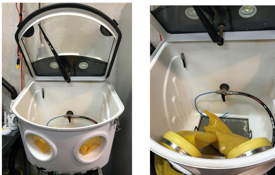
Figure 25: Photograph of the power washing station used to remove Objet Support SUP707 material from samples printed using PolyJet technology.
