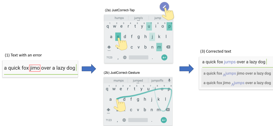
Figure 4.11: (1) The user enters a sentence with an error jimo using tap typing; (2) To correct jimo to jumps , they can either tap-type jumps and press the editing button (2a), or switch to gesture type jumps (2b). (3) JustCorrect then substitutes jimo with jumps . Two alternative correction options are also presented. The editing procedure involves no manual operations except entering the correct text.
