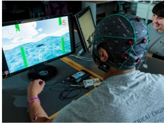
Figure 3.4: A subject plays the computer game Flappy Whale. The electrode recording muscle electrical activity (that controls the whale) can be seen on the subject's left arm.
