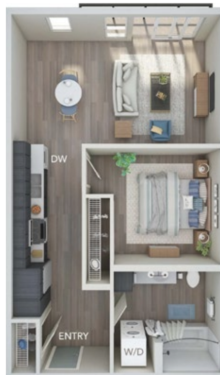
Figure 7: A typical single aspect, “one bedroom” apartment layout from new construction in Seattle showing a narrow, deep unit (Hemlock, n.d.).
