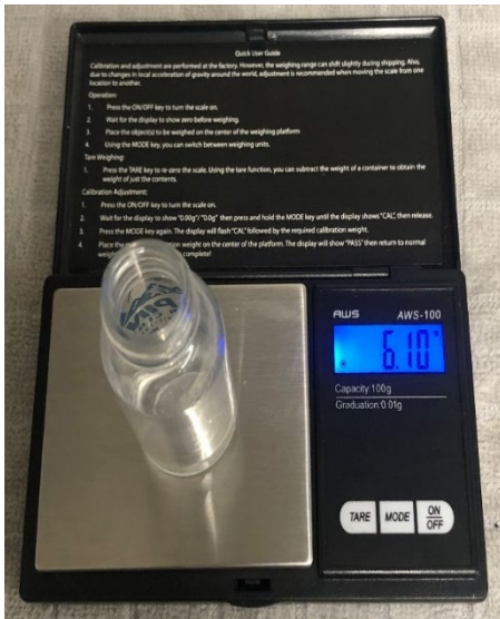
Figure B 3 Example of controlling the amount of liquid deicer in the spray
