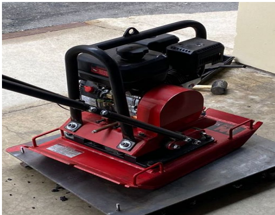
Figure 3.1 Plate compactor and asphalt test slab prepared in the study
