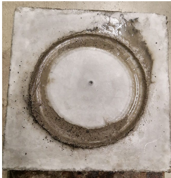
Figure 3.8 Concrete slabs tested with the TWPD
