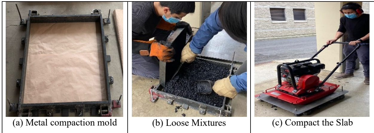
Figure A1. Preparation and compaction of the test slabs
