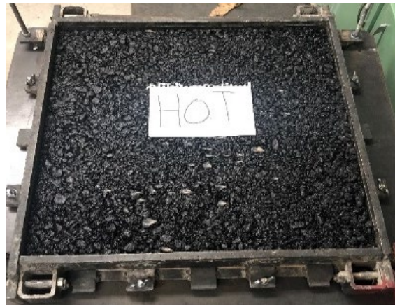
Figure 3.1 Plate compactor and asphalt test slab prepared in the study
