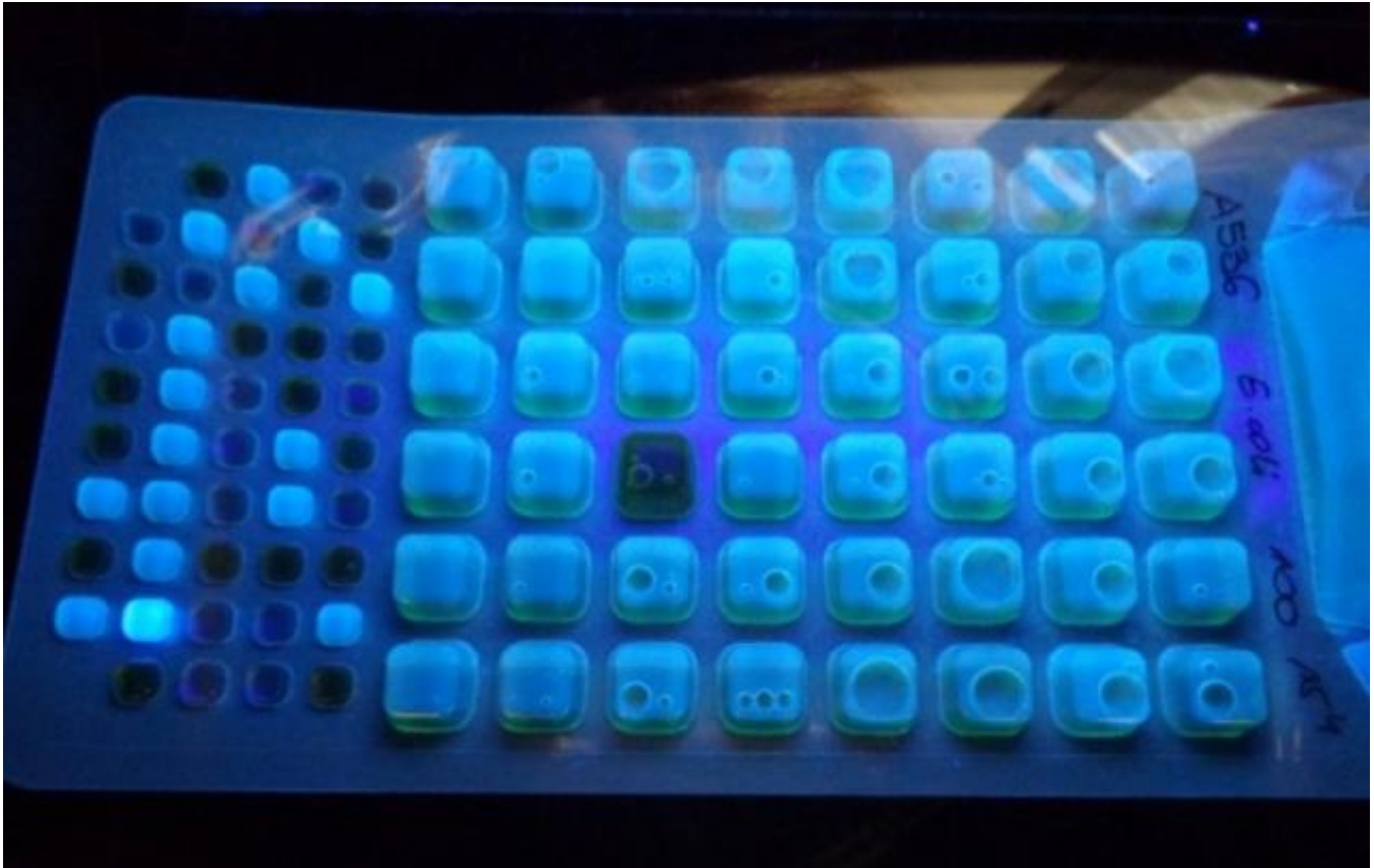
Figure 5. Quanti-Tray 2000 under UV light indicating florescent cells, some with gas formation, that are positive for MUG metabolism.
