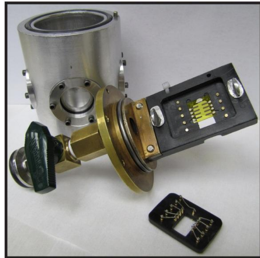
Figure A-2: (Top) The custom-built electroabsorption apparatus. (Bottom left) Close-up of the vacuum test chamber, showing the geometry of the optical probe and detection. (Bottom right) Device holder with 8-pixel Super Yellow diode chip.
