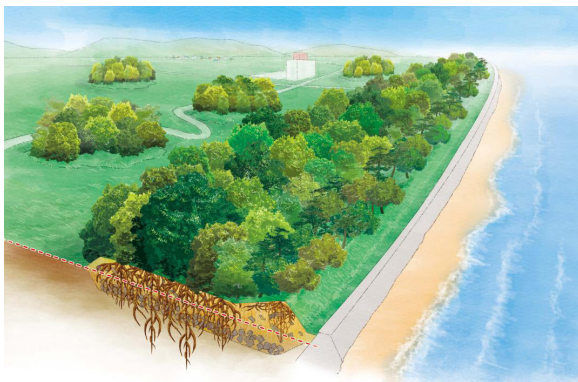
Figure 37. A rendering that shows a hybrid mitigation park layout with a coastal forest and sea wall. Image by PUR Project ( Morino Project 2016).
