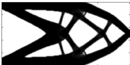
SIMP, 50 Iterations, \bar{f} = 63.4
