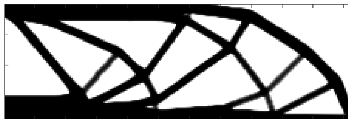
Figure 4.30. Reference manufacturable SIMP solution, 1200 iterations, minimum element thickness of 1.0mm. \bar{f} = 219.43
