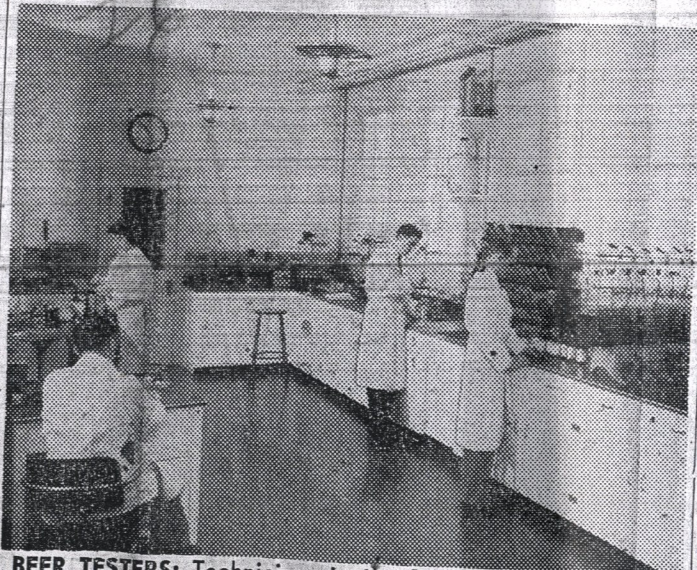
BEER TESTERS: Technicians in the Rainier laboratory subject every batch of beer to a variety of chemical tests to assure uniform quality.
