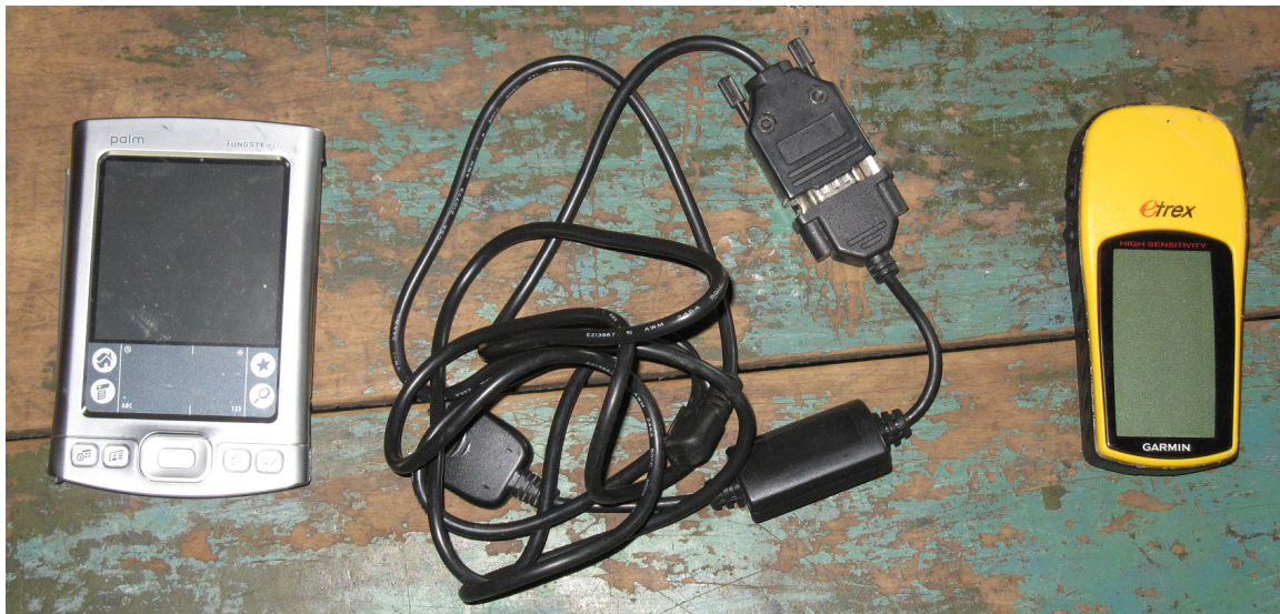
Figure 5.2: Palm TX, eTrex GPS, and connecting cable used by AMPATH prior to implementing a system with ODK.
