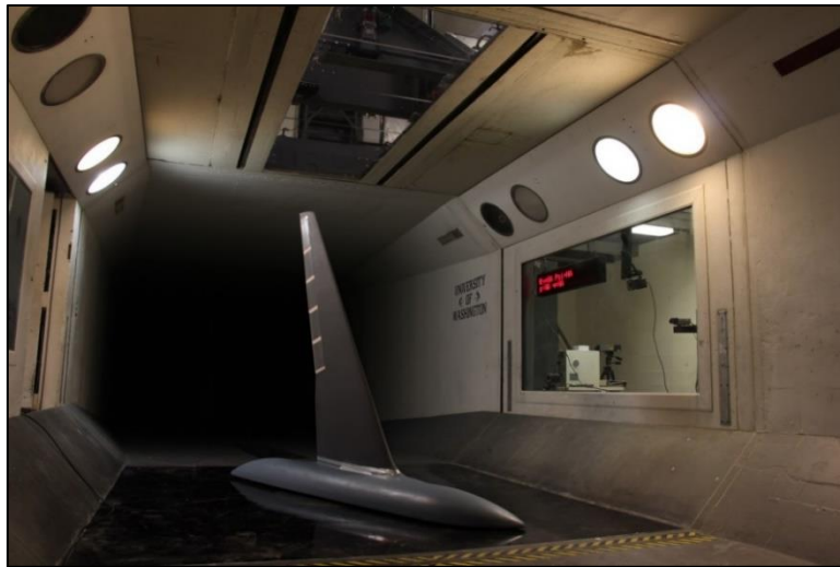
Figure 1: Front view of the clean wing GTM VCCTEF aeroelastic model at the KWT
