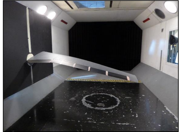
Figure 7: The wing on the sidewall balance next to the boundary layer splitter plate – rear view
