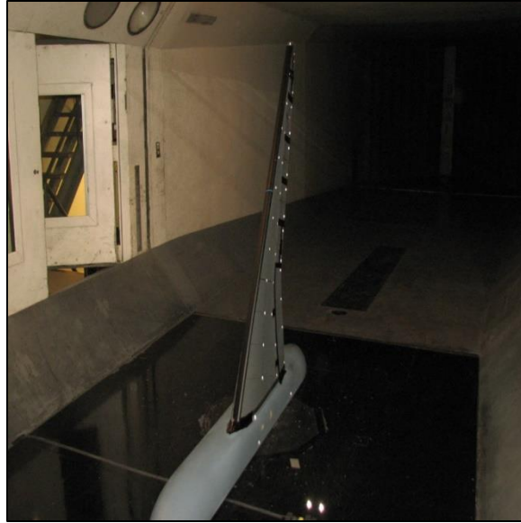
Figure 2: The high-lift GTM based VCCTEF aeroelastic wing model at the KWT
