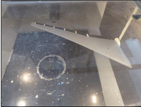
Figure 6: The wing on the sidewall balance next to the boundary layer splitter plate – top view
