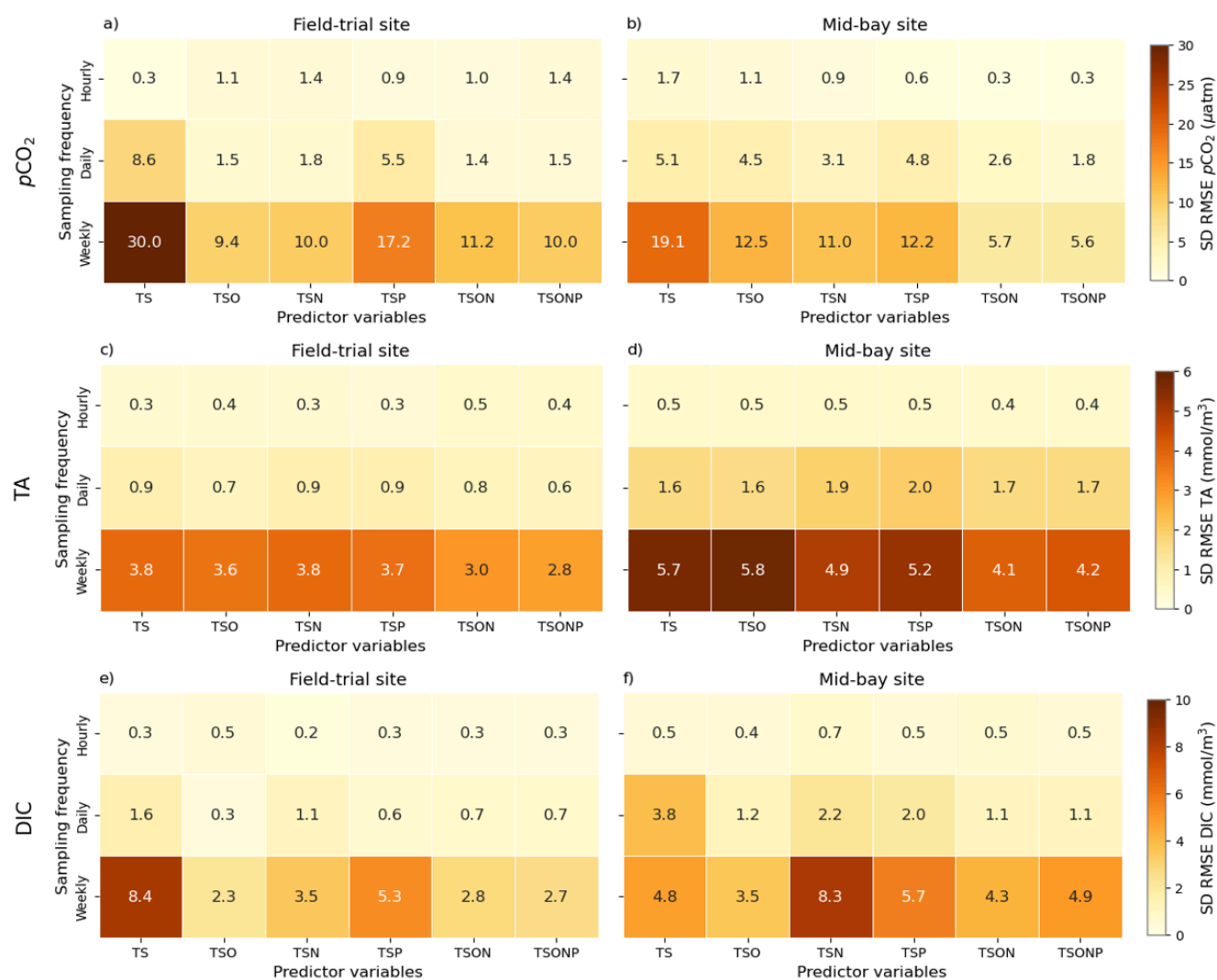
Figure S4| Standard deviation (SD) of RMSE from five-fold cross-validation of predictive algorithms at the field-trial (a, c, e) and mid-bay (b, d, f) sites. Each panel presents a heat-map table of the standard deviation of RMSE values from five-fold cross validations, calculated at three sampling frequencies (hourly, daily, weekly) for three carbonate chemistry variables: p\text{CO}_2 (a–b), TA (c–d), and DIC (e–f). The columns correspond to different combinations of predictor variables ( TS , TSO , TSN , TSP , TSON , and TSONP ). Lower standard deviations indicate more precise algorithm performance.
