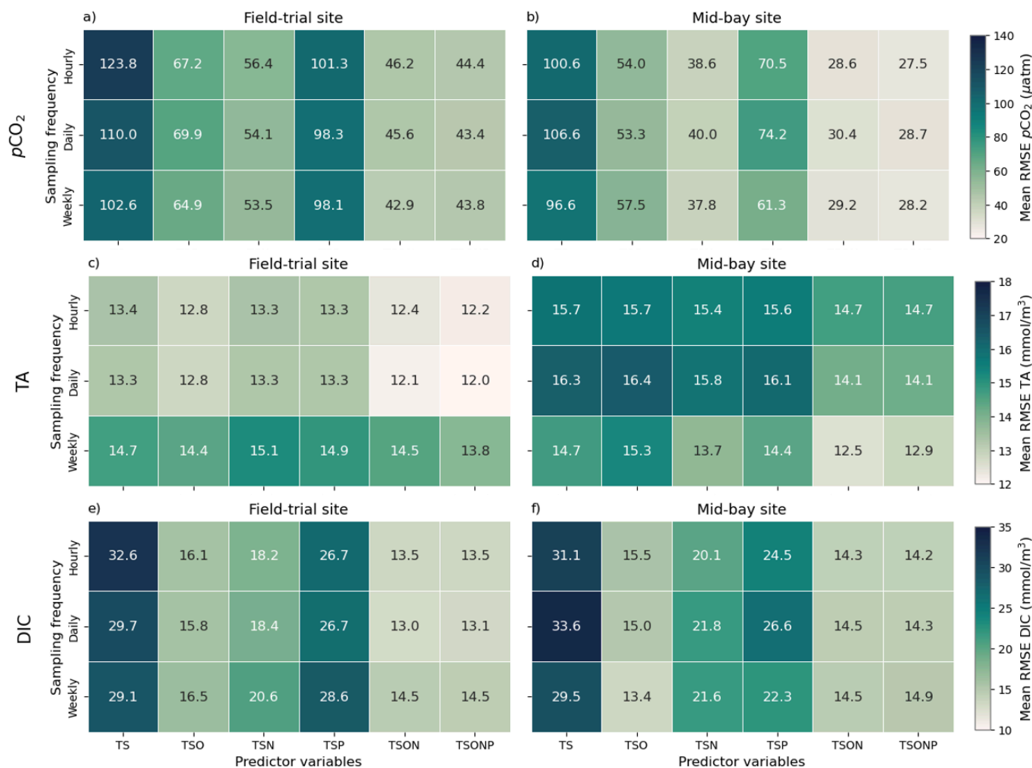
Figure S3| Mean RMSE from five-fold cross-validation of predictive algorithms at the field-trial (a, c, e) and mid-bay (b, d, f) sites. Each panel shows a heat-map table of mean RMSE values from five-fold cross validations, calculated at three sampling frequencies (hourly, daily, weekly) for three carbonate chemistry variables: p\text{CO}_2 (a–b), TA (c–d), and DIC (e–f). The columns correspond to different combinations of predictor variables ( TS , TSO , TSN , TSP , TSON , and TSONP ). Lower RMSE values denote better algorithm performance.
