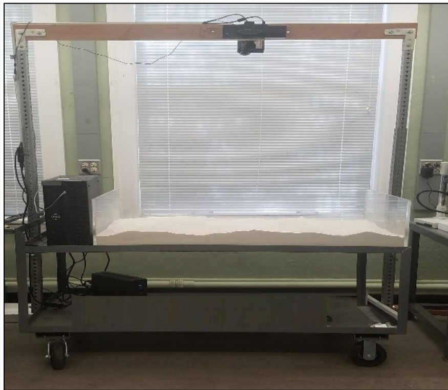
Figure 3-12. Schematic diagram of the AR sandbox
