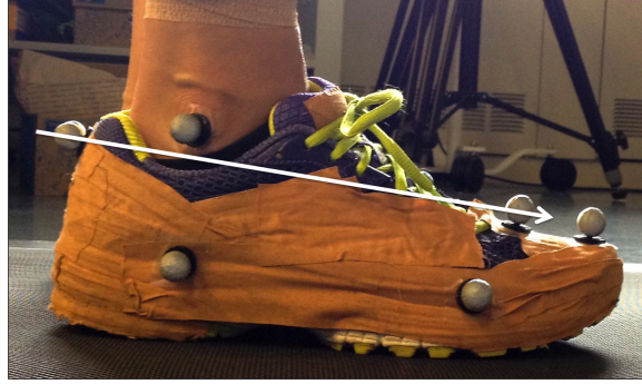
Figure 3.14: Retro-reflective marker placement on right foot and vector for foot strike angle calculation.
