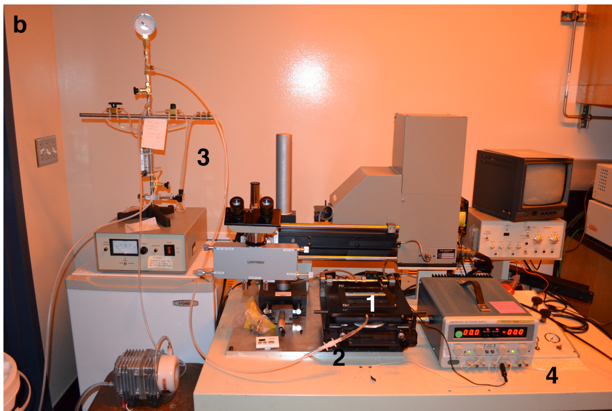
Figure 5.7. Gold-coated PDMS stamped fabricated from an entire CD (a). Schematic of wafer-scale reactive stamping prototype (b), including mounting of wafer-scale stamp (b1), retrofitting gas purge lines (b2,3), and application of an external voltage (b4).
