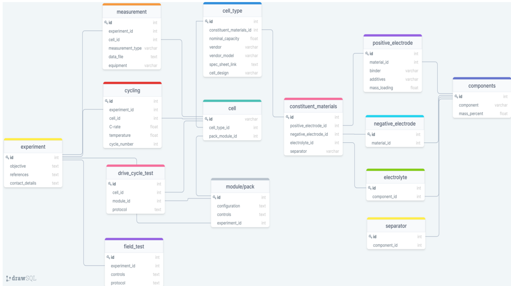
Figure 4.11: Proposed schema from the Battery Genome Group. This includes primary, secondary, and tertiary metadata.
