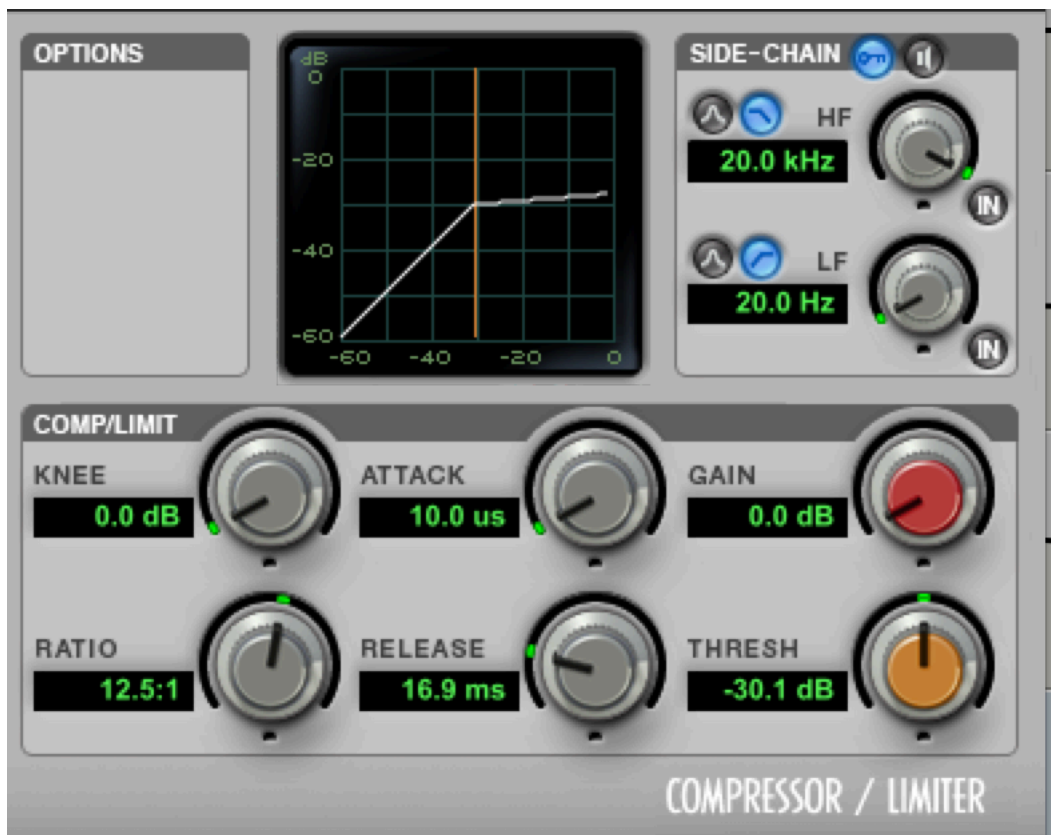
Sub compressor sidechained from Kick (Fig. 27)
