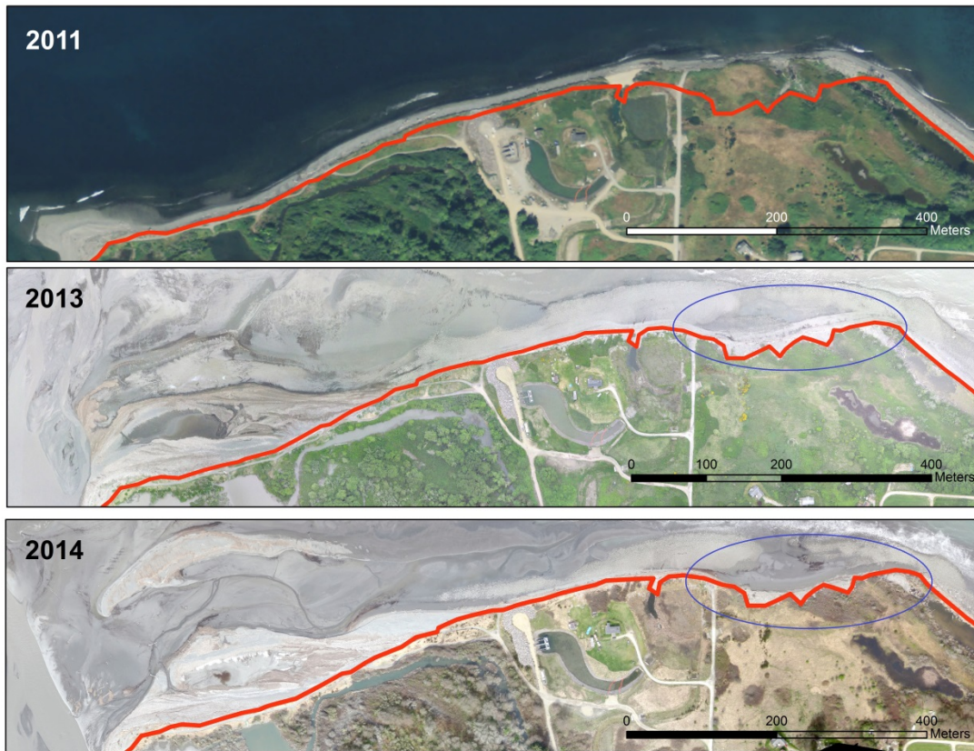
Figure 9. Shoreline evolution east of the river mouth during dam removal. The 2014 vegetation line is marked in red on all three panels. Note the shoreline region circled in blue where sediment resembling the accretion at the river mouth has deposited on top of vegetation between 2013 and 2014. Aerial photograph credits: U.S. Department of Agriculture (2011); Andy Ritchie, National Park Service (2013, 2014)
