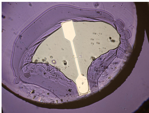
Figure 2.5: The fabrication process of a graphene + hBN device. See the main text for description. Newton's rings form as the stamp comes in contact with the substrate.
